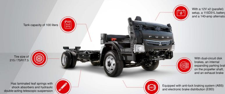
With a 12V x2 (parallel) setup, a 115D31L battery, and a 140-amp alternator
