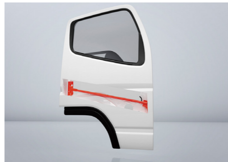
Side impact beams built into the doors strengthening door frame and rigidity to protect the driver and passengers.
