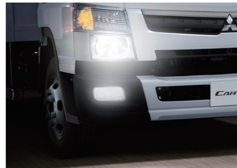
Bright, twin-bulb, adjustable halogen headlamps and fog lamps come standard for safer driving conditions.
