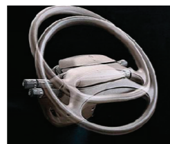
Tilt adjustable steering wheel with collapsible steering column
