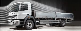
The FJ's aerodynamic cab design reduces wind resistance thus reducing cabin noise while increasing fuel efficiency
