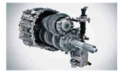
The Fuso FJ is equipped with a smooth-shifting 9-speed manual transmission which provides a higher flexibility of gear selection for various operating conditions thereby enhancing driving performance and improving fuel efficiency
