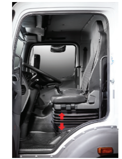
The multi-adjustable air pressure driver's seat and tilt and telescopic adjustable steering wheel allow the driver to set the optimum driving position for comfort and performance.
