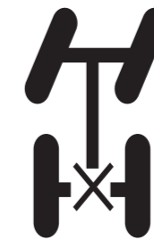
The Differential Lock Buzzer informs driver of differential lock position
