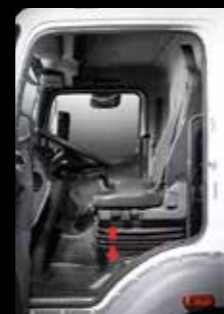
The multi-adjustable air pressure driver's seat and tilt and telescopic adjustable steering wheel allow the driver to set the optimum driving position.
