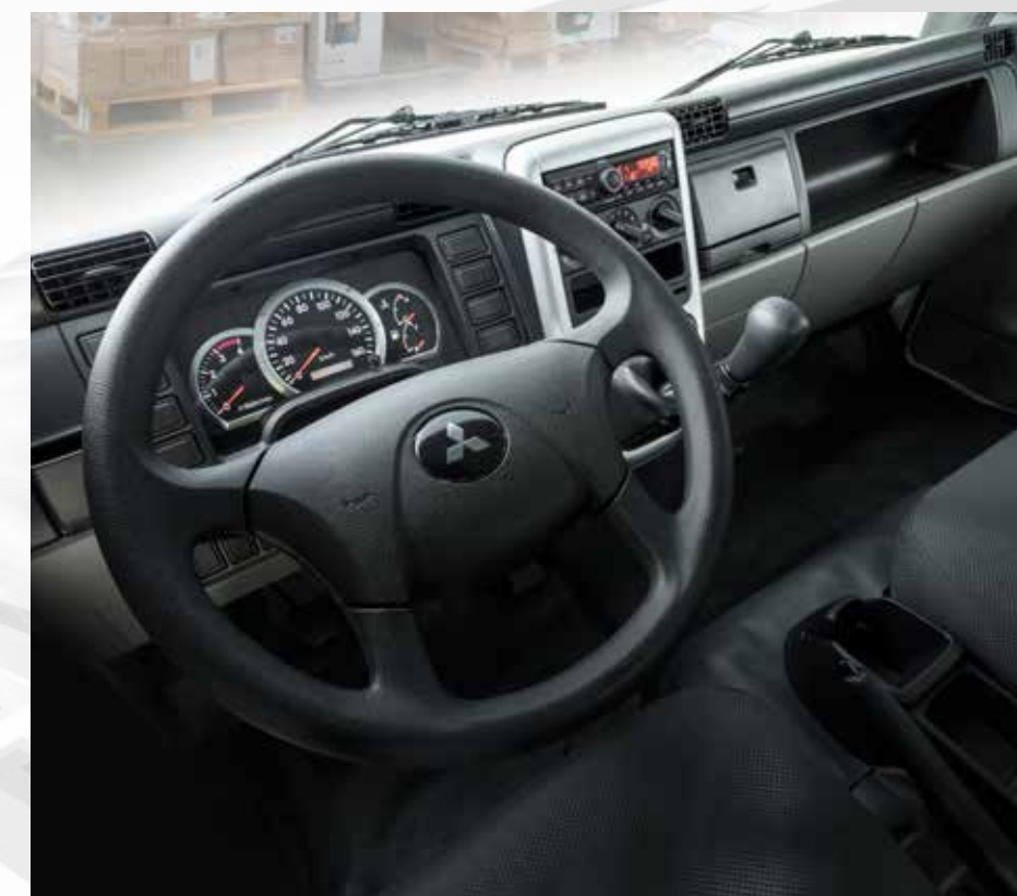
The tilt & telescopic adjustable steering wheel and dash-mounted gear shift location allows for the best driving position. (Audio head unit is customer option.)
